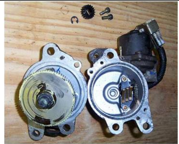
Figure 6. Front actuator internals
