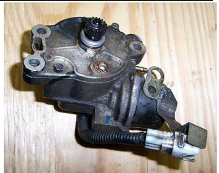
Figure 3. Front differential lock actuator
