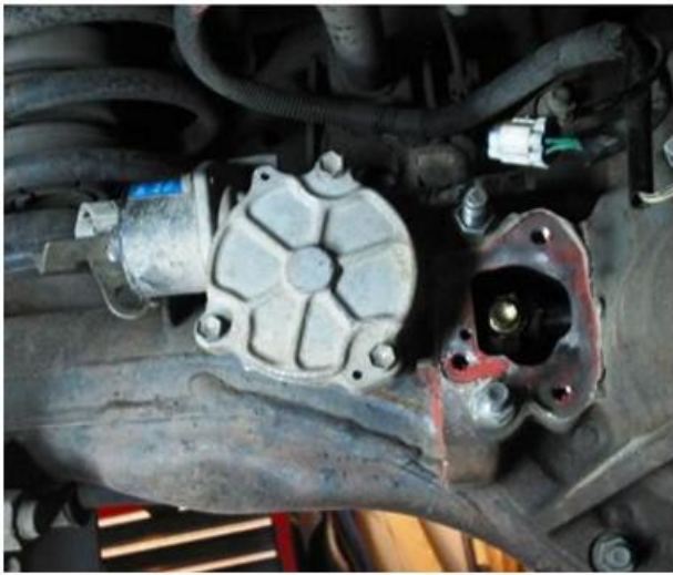
Figure 1. Rear locker actuator with axle cover plate removed, exposing shift fork connection.
