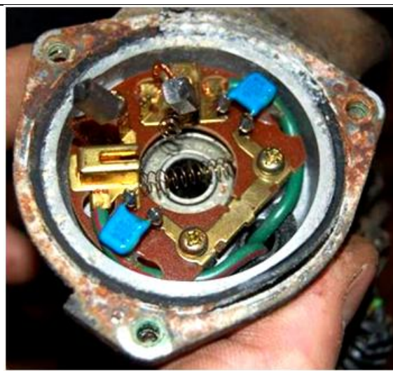
Figure 8. Springs and brushes after motor armature removal
