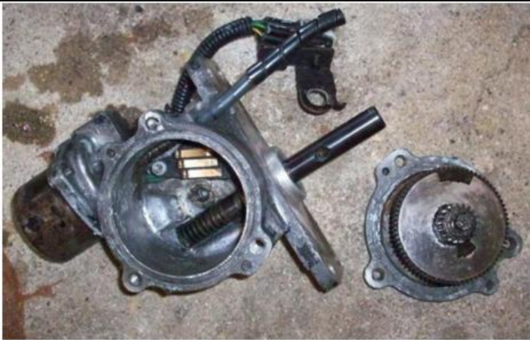
Figure 5. Rear actuator internals
