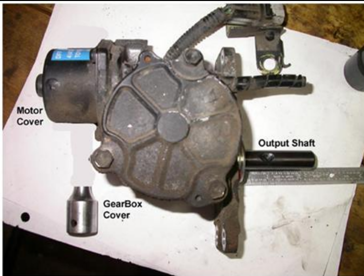
Figure 2. Rear differential lock actuator
